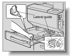
4 For Over Size Paper, adjust the trailing-edge guides as shown in the illustration.
